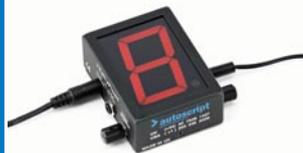
TallyPlus is a unique camera number system. A large LED indicator displays the number in green (1-9) while in standby, then turns red when the camera is live. Switching from green to red is achieved by a photo electric cell that can be attached to the camera tally light. TallyPlus retrofits to the whole range of Autoscript TFTs and has the unique feature of a second photo electric cell built into the rear of TallyPlus that docks with the cue light on the TFT.
