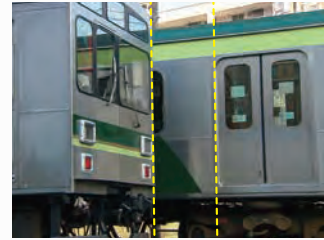
No Rolling Shutter Artifacts with Global Shutter
