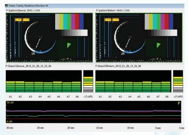
The RTM 4K presents a significant technological breakthrough by applying a fully uncompressed 4K video source with embedded audio and performing a real-time video PSNR or DMOS via comparison to a 4K encoded/decoded signal input along with audio quality, lip sync and audio program loudness measurements at the same time.
