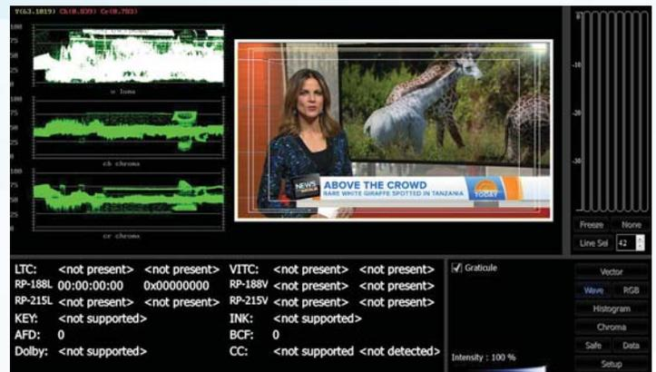
**Signal Compare** - Used to freeze a complete frame of video (two fields in interlaced), every second line (field) or at a 50/50 dissolve to compare two signals or cameras.
