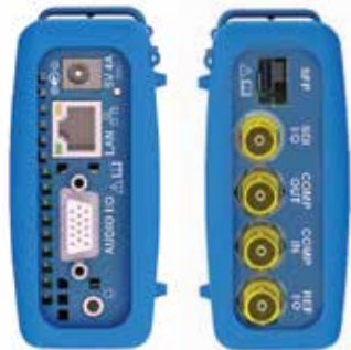
DC 5V power & recharge Ethernet Headphone Composite In/Out, HD, SD SDI In or Out Bi/Tri-level Reference In/Out SFP cage
